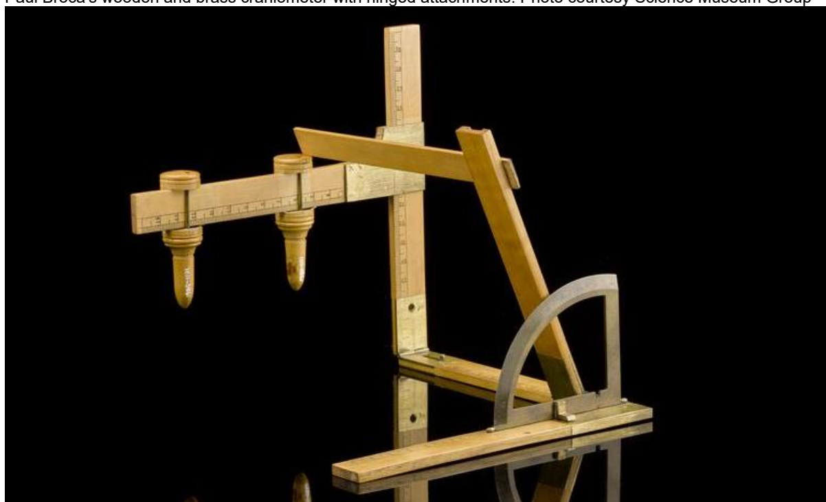
Broca goniometer for determining the 'facial angle.' Photo courtesy Science Museum Group
